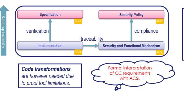
Bottom-up approach intrinsically encompasses the refinement from the security and functional specifications through the design to the implementation.
